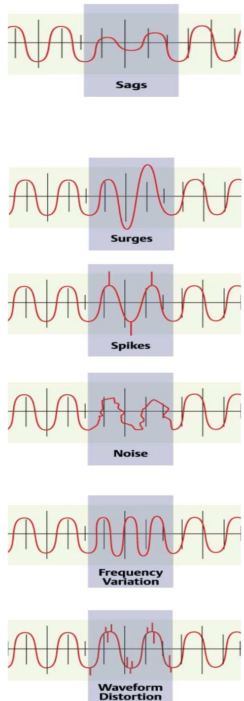
**Figure 2. System protection must be ready to handle a wide array of power fluctuations. The illustrations show waveforms for typical 60 Hz AC power. The left and right unshaded areas show how the waveform should look; the shaded area shows how the disturbance distorts the waveform.**
